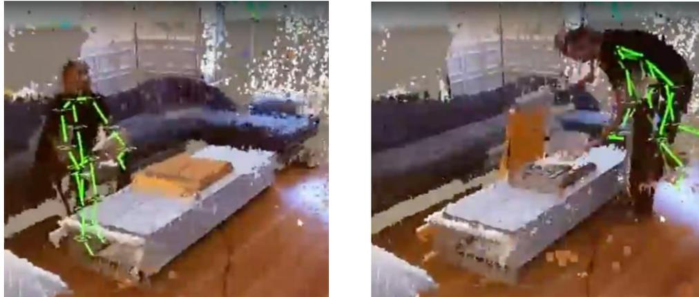
*Fig. 2. Top: Volumetric capture using Kinect depth sensors without (left) and with (right) human motion tracking. Captured as it is shown in XR (Varjo VR-2 Pro headset). Bottom: Volumetric capture detecting the skeleton of human body and its joint points (Varjo VR-2 Pro headset).*
