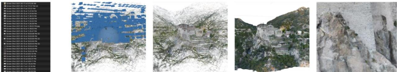
data input: images → photo alignment → point-cloud → mesh object → texture mapping
