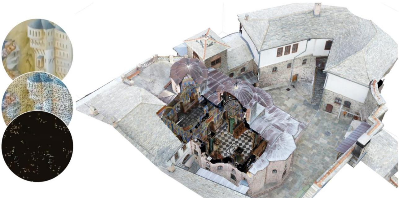
Fig. 1. Top: Steps of post-processing photogrammetry data in Agisoft Metashape – technique A (see text). Bottom Left: tie-points, point-cloud, 3D geometry with texture mapping of the main church interior space. Bottom Right: Perspectival view of Simonos Petra main courtyard and partially revealed the main church space.
