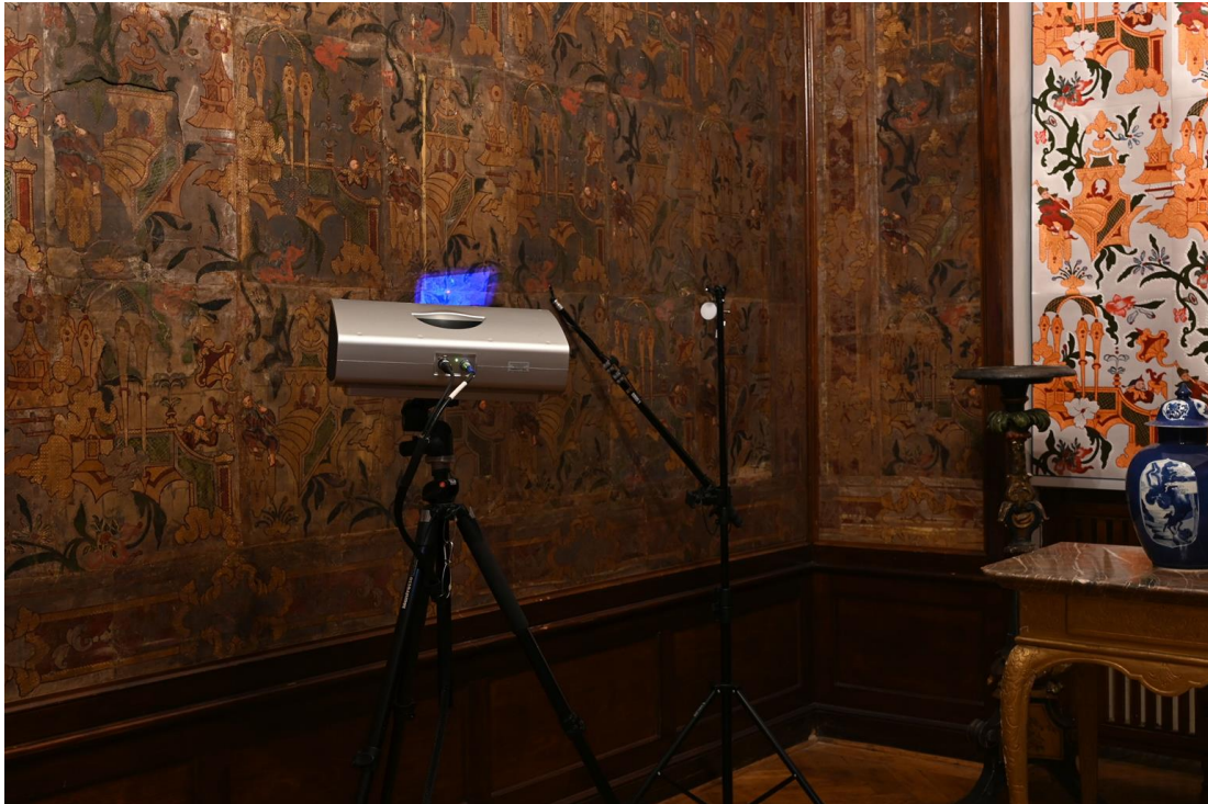
Fig. 1. Examination of the leather panels in the Chinese room in Moritzburg Castle with the COMET L3D 5M. Next to it, the microclimate (surface temperature, relative humidity, and temperature) is measured (© Kristina Holl).
