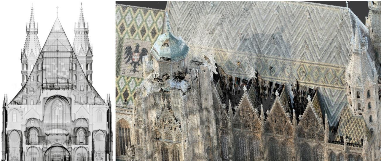
Fig. 1. Different renderings of TLS-point-cloud. Left: X-ray view along main axis of the cathedral making structures orthogonal to the viewing direction visible (black) while structures parallel to the projection plane become transparent. Right: Coloured TLS-point-cloud of high up regions showing shadowed (i.e. invisible) areas.
