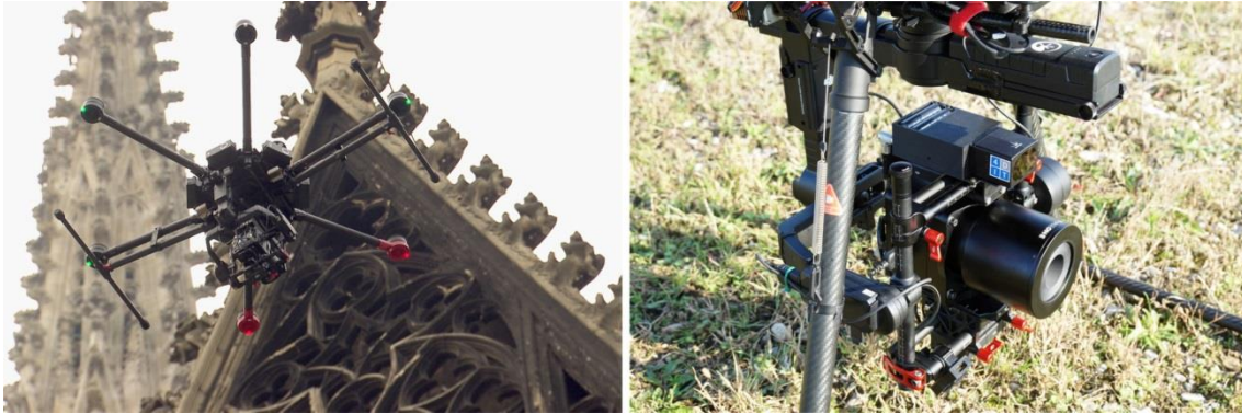
Fig. 2. UAV flight at St. Stephen's was realized with a DJI Matrice 600 pro and Phase One iXM 100 camera with RSM 80 mm AF lens and 4DU-RangeFinder. The system during data acquisition is shown left and the sensor system right.
