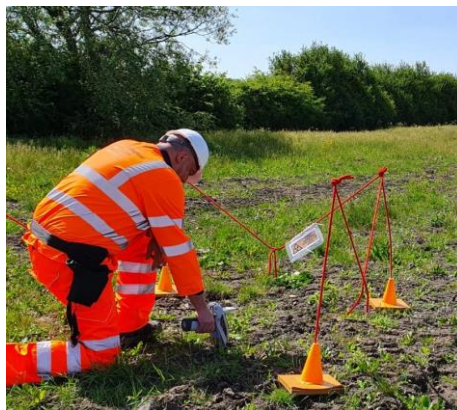
Figure 1. A geochemical analysis being undertaken in the field using a portable XRF instrument (© Fusion JV).
