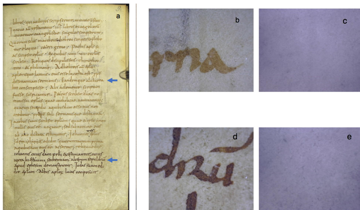
Fig. 4. Cod. 808, fol. 9r with two seemingly different inks. Blue arrow indicates the letters shown in the micrographs on the right, b & d are taken under visible, c & e – under NIR illumination
