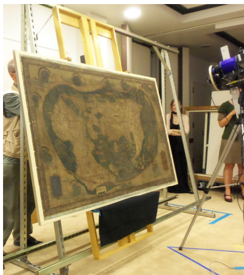
Fig. 2. Martellus map mounted on moveable easel with Megavision E7 camera
