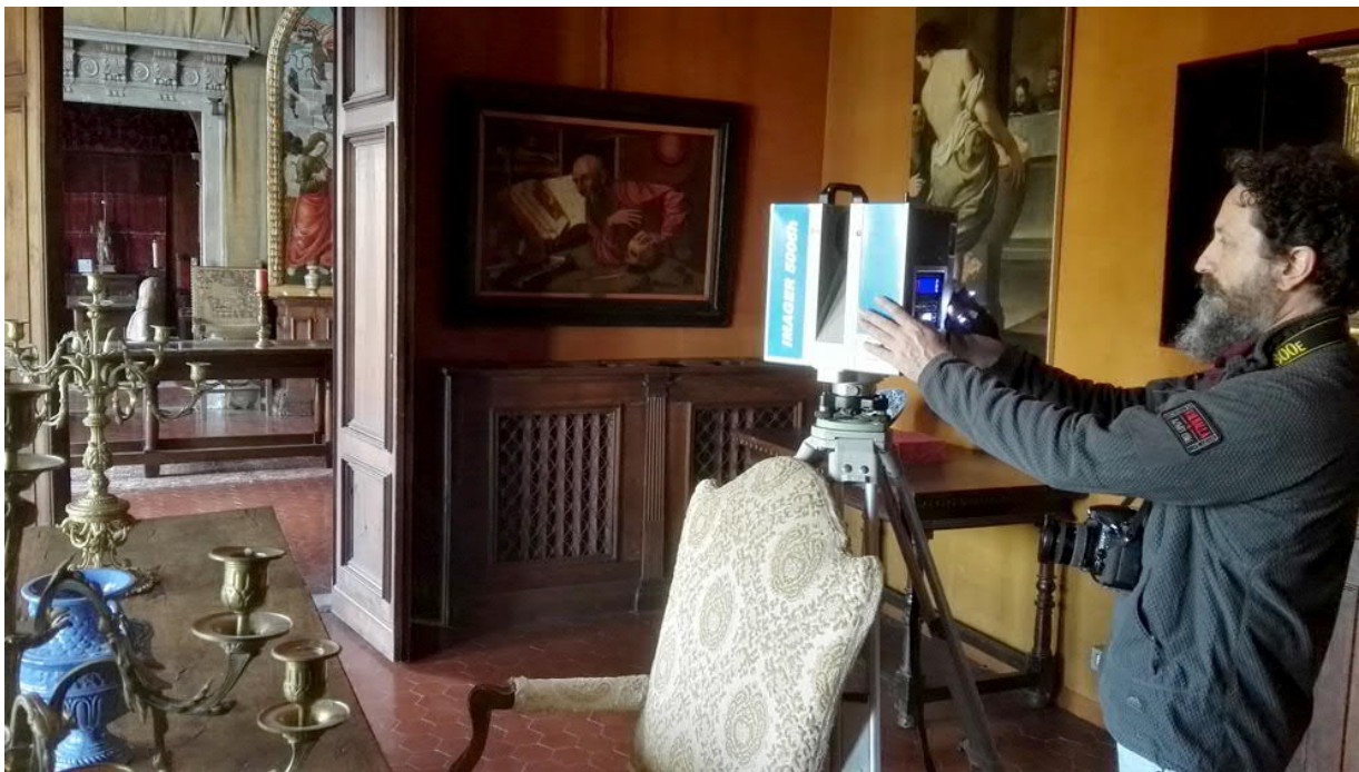
Fig. 6. The campaign carried out with 3D Laser Scanner on the Gallery's first floor
