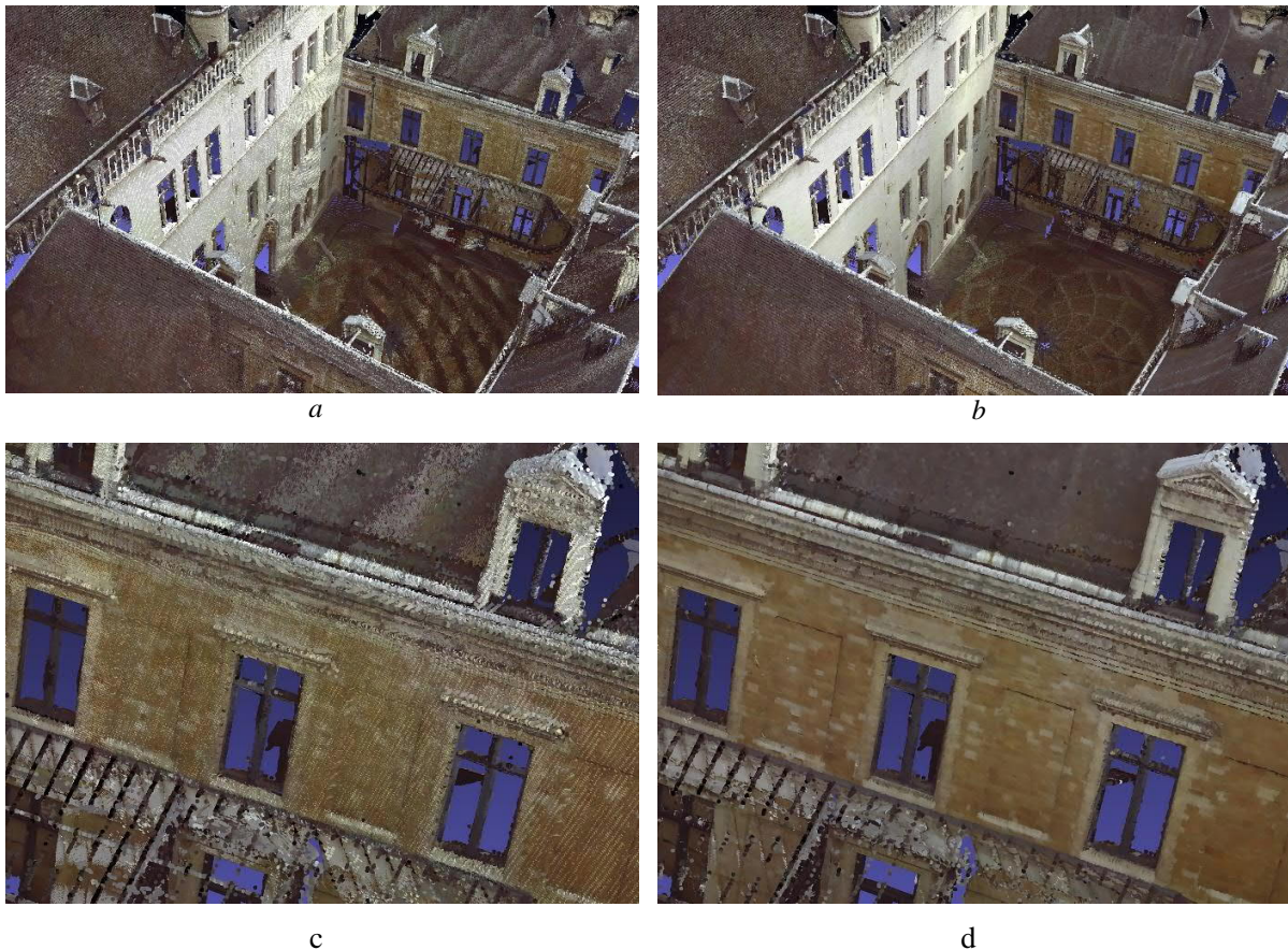
Fig. 5. Example of color correction for the City Hall Courtyard: a) & c) Raw points cloud, b) & d) Corrected colors model
