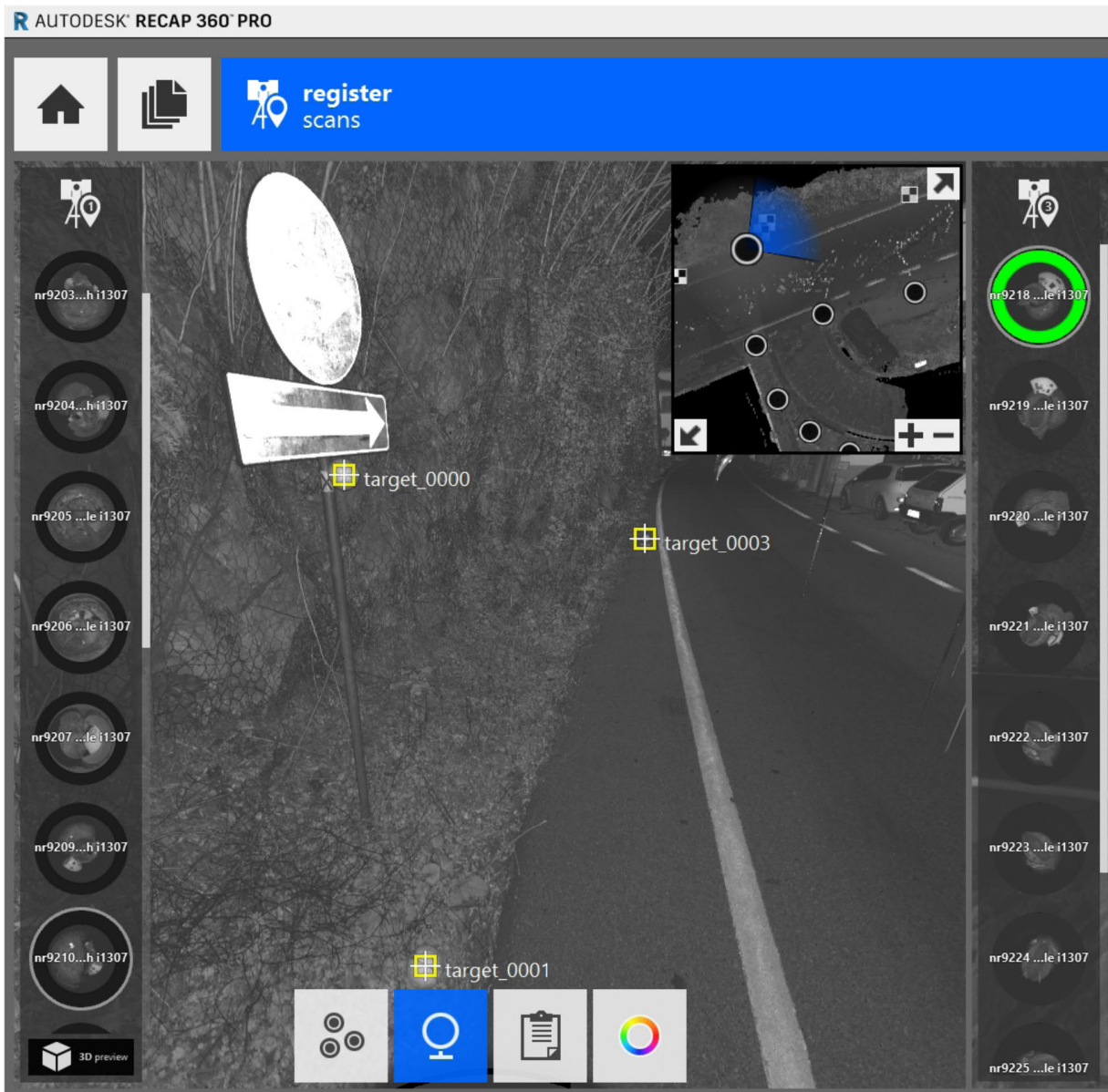
Fig. 4. Screenshot of Autodesk ReCap Pro. Target detection
