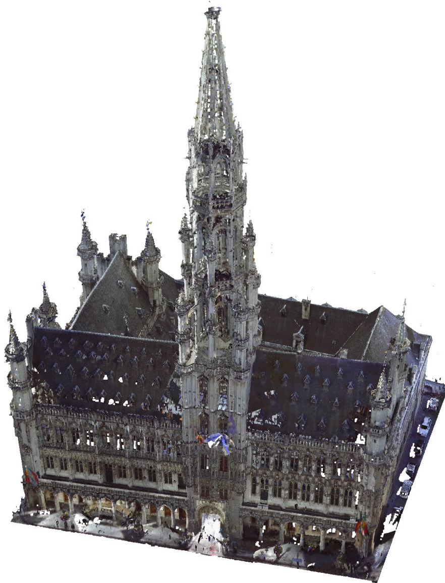
Fig. 2. Point cloud of the Brussels City Hall acquired with a Faro S120 3D Scanner
