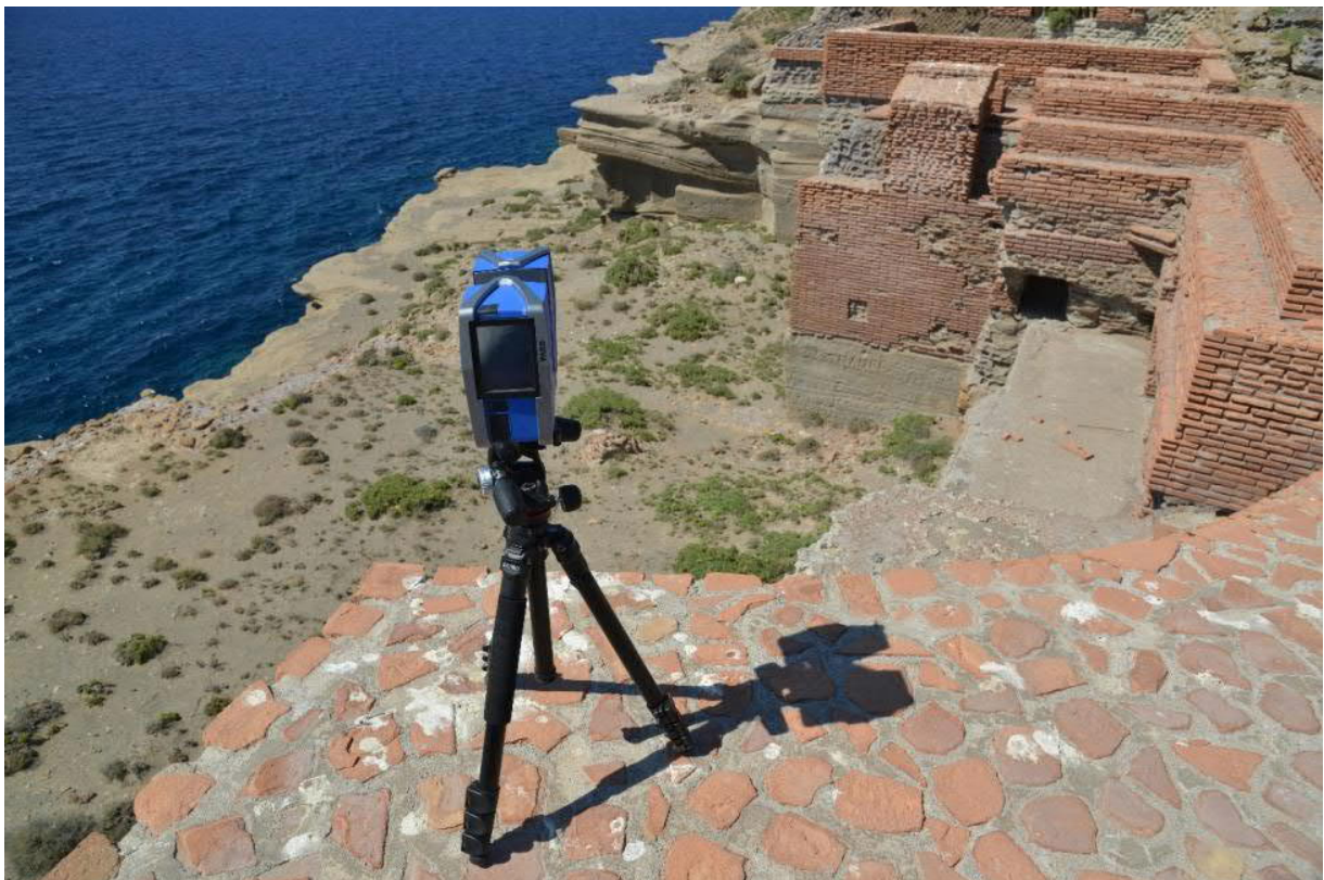
Fig. 8. 3D laser scanner Faro X 330
