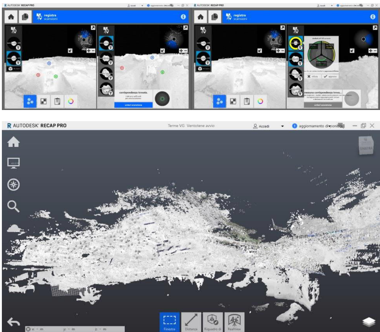
Figs. 9-10. Scanner recorder operations (top) and final 3D cloud (bottom)
