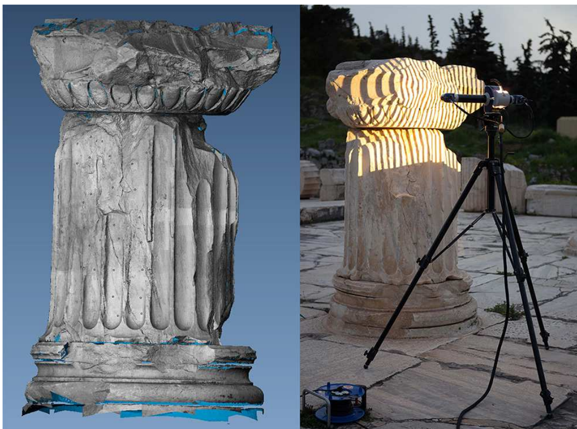
Fig. 8 – Visualisation of the 3D scanning results from Elefsis in OPTOCAT software (left). Data acquisition with a Beuckmann white light scanning system (right).
