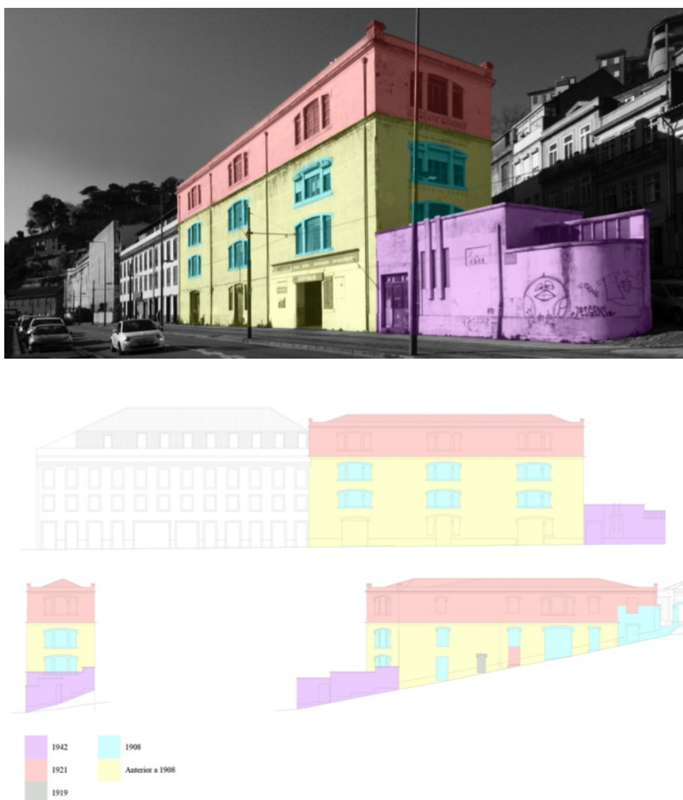
Fig. 1. Stratigraphic reading of one of the sectors of the convent. Photomontage and elevations. Self elaboration. 2019.
