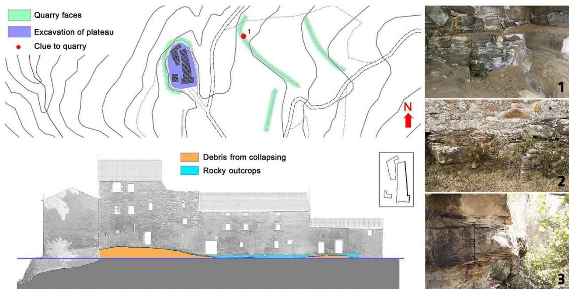
Fig. 9 – The geological analysis allowed to verify that the material with which the whole town was built comes from the same geological area, so it seemed logical to look for a possible quarry in the vicinity of the castle: 1. Internal masonry on rocky outcrop, 2. Outcrops on East side of the settlement, 3. Metric verification of the origin of the stones (S. Di Grazia)
