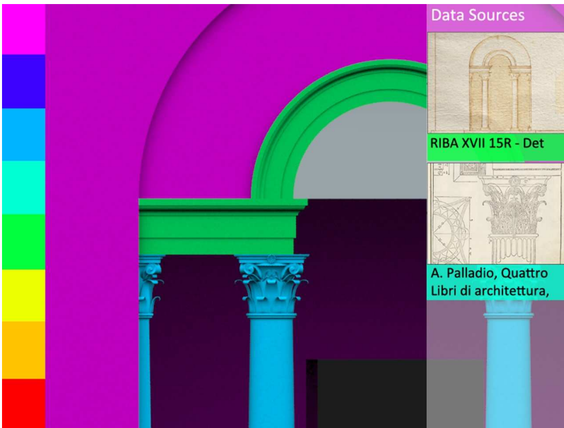
Fig. 4 – A. Palladio, ‘Villa for a twin’. 3D Virtual Reconstruction after RIBA XVII 15R. Detail of loggia with Serliana and Corinthian order: displaying uncertainty of reconstructive hypotheses based on different data sources.
