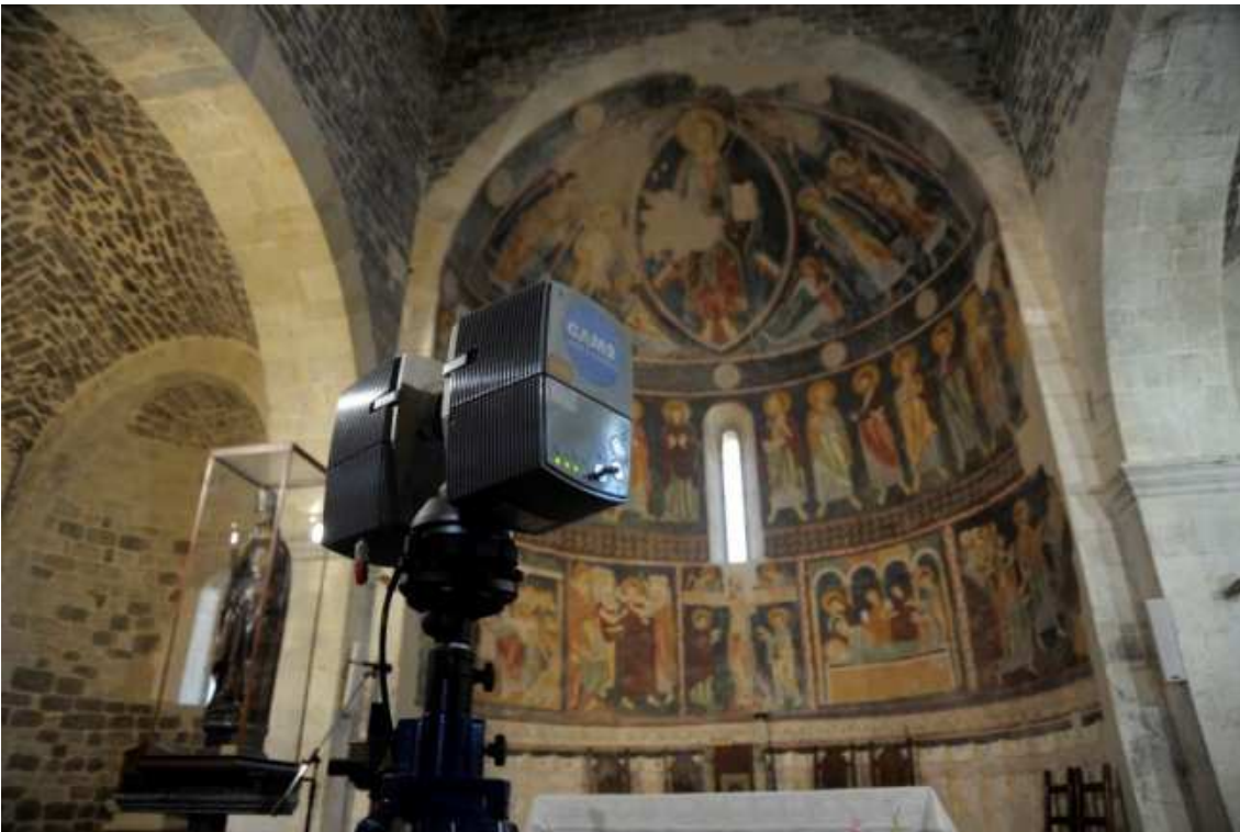
Fig. 7 – 3D CAM/2 Faro Photon Laser Scanner. (Copyright: Giorgio Verdiani)
