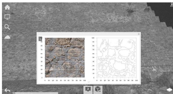
Fig. 18. Insertion of masonry survey into the point cloud - Venetian Masonry (1489-1570)
