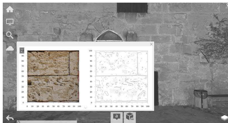
Fig. 15. Insertion of masonry survey into the point cloud - Lusignan Masonry (1192-1489)
