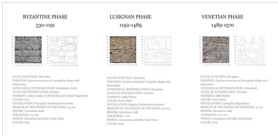
Fig. 9. Masonry survey of Kyrenia Castle (© E. Valletta)
