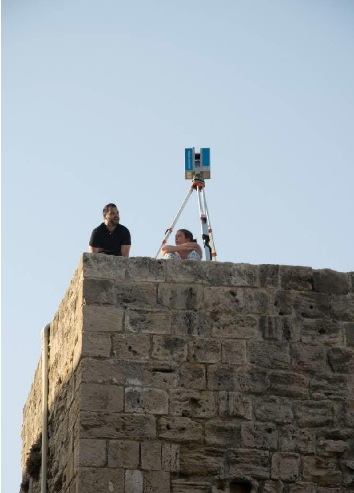
Fig. 2. Laser scanner survey: digital data gathering (© G. Verdiani)
