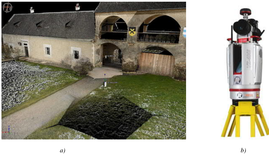
Fig. 3. a) Two colored laser scans, distance between the scan positions approx. 10 meters; b) RIEGL VZ-400i terrestrial laser scanner combined with a Nikon D-810 digital camera and a GNSS receiver
