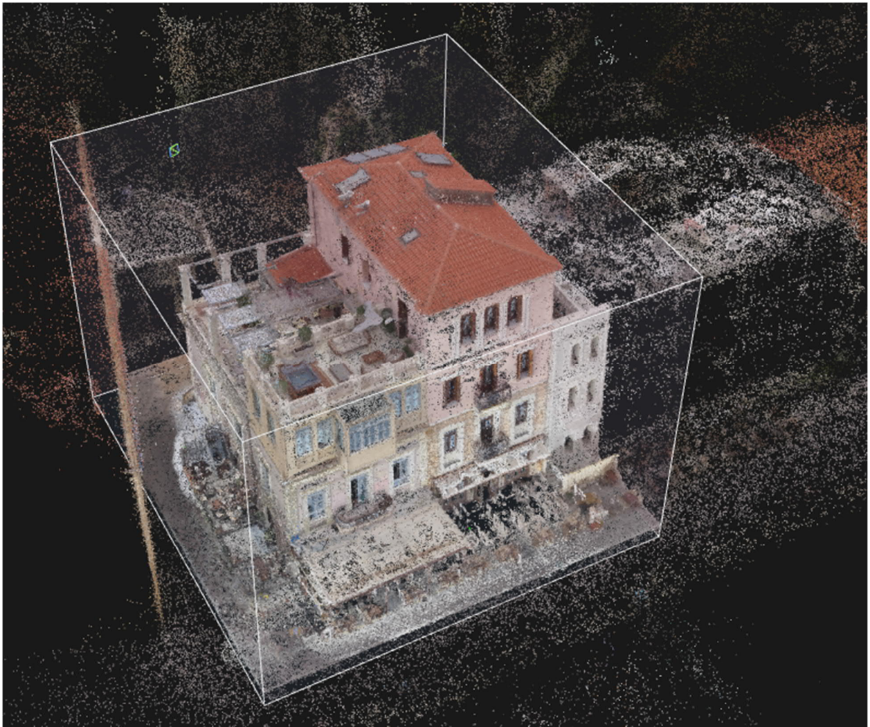
Fig. 5. 3D Point Cloud in Reality Capture
