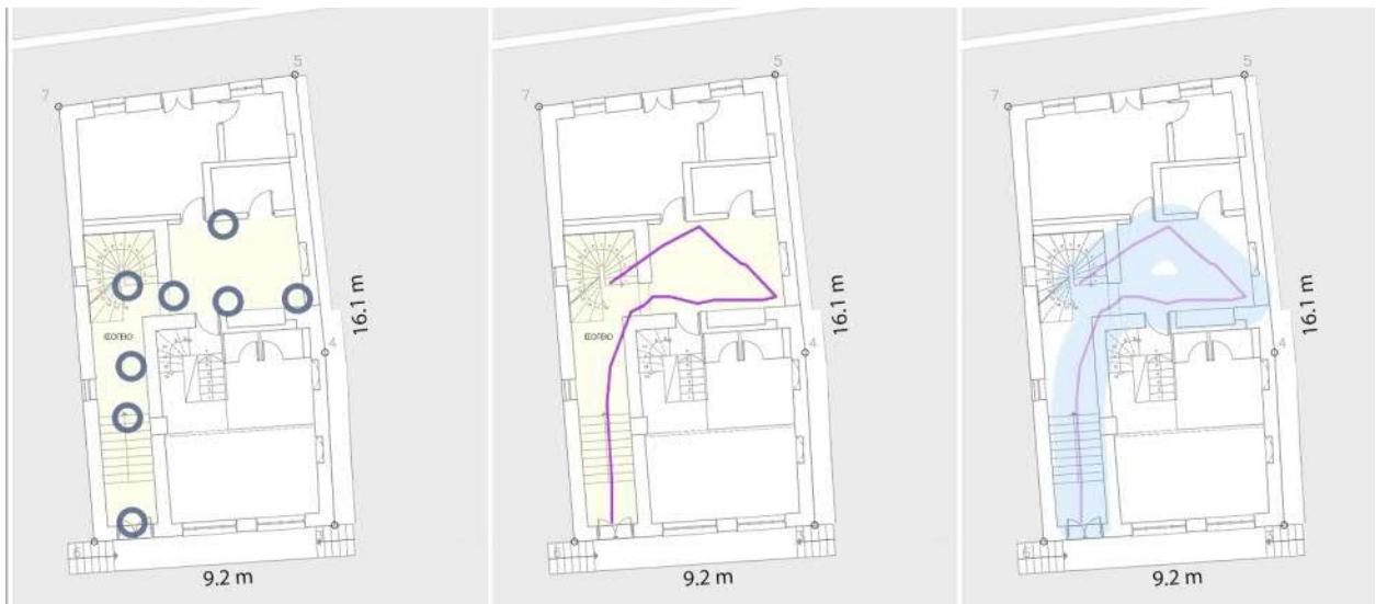
Fig. 8. Mapping process a) insertion of waypoints; b) creation of path; c) creation of digital map
