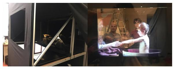
Fig. 3. a) Lateral picture of the holographic showcase with 45° glass, back objects and frontal glass clearly visible; b) effect produced by the transparent glass at the back of the structure
