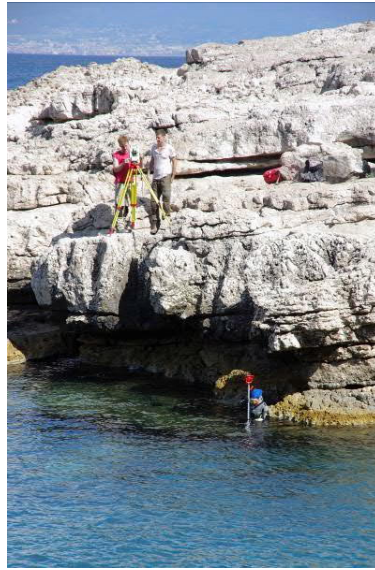
Fig. 3. Documentation of submerged structures with the total station (© G. Graf)
