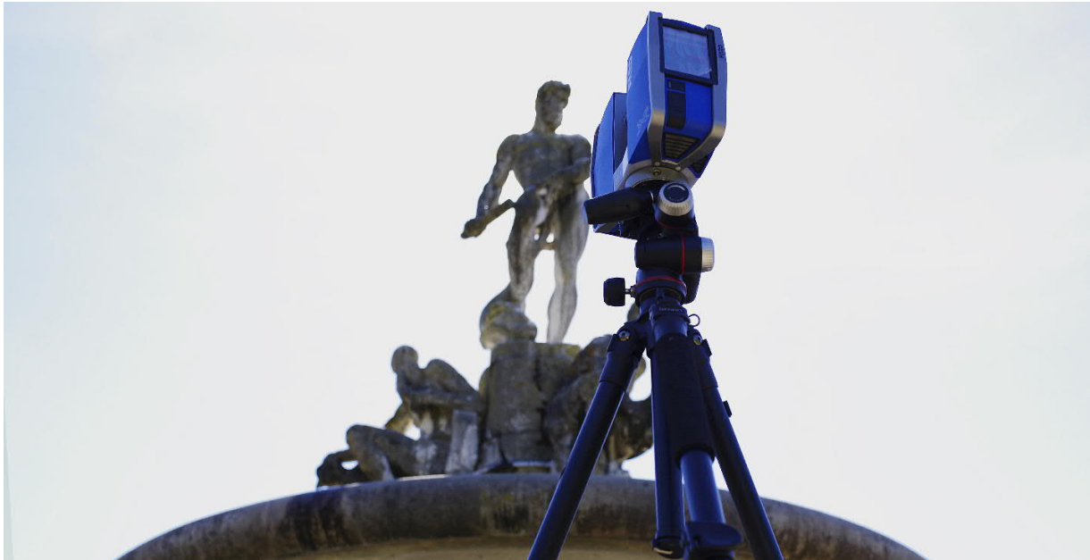
Fig. 9. 3D Laser scanner survey of the “Fountain of the island” in the Boboli Garden
